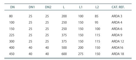
DN1 is used for insertion of a thermometer pocket. DN2 is recommended on the distillate outlet.
